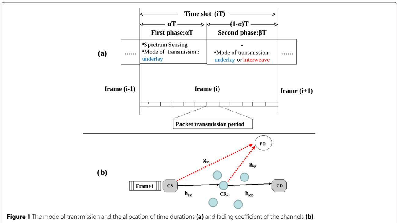
**Figure 1** The mode of transmission and the allocation of time durations (a) and fading coefficient of the channels (b).
