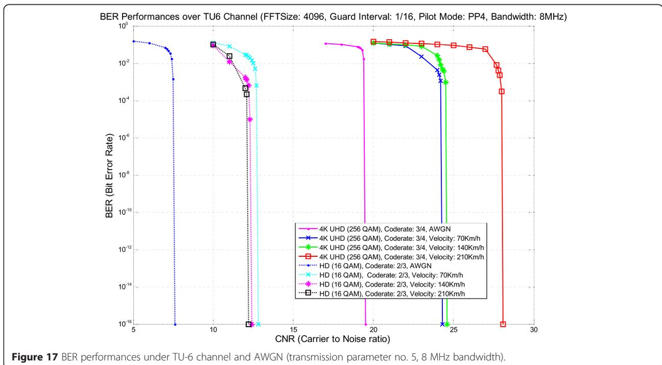
**Figure 17** BER performances under TU-6 channel and AWGN (transmission parameter no. 5, 8 MHz bandwidth).
