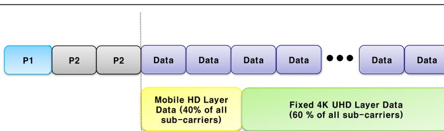
**Figure 8** Transmission frame structure for terrestrial 4 K UHD and HD convergence broadcasting.
