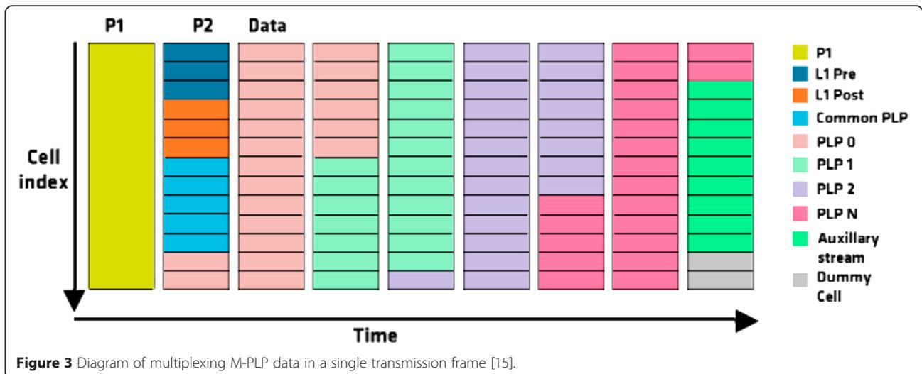
**Figure 3** Diagram of multiplexing M-PLP data in a single transmission frame [15].
