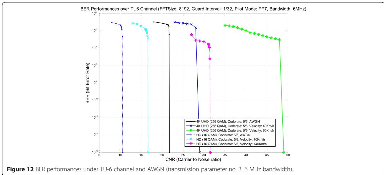
**Figure 12** BER performances under TU-6 channel and AWGN (transmission parameter no. 3, 6 MHz bandwidth).
