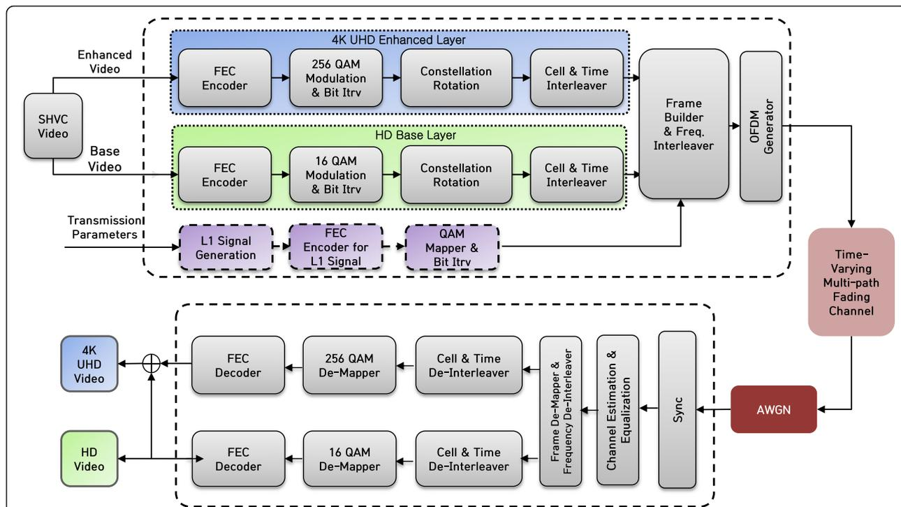
Figure 7 Structure of terrestrial 4 K UHD and HD convergence broadcasting transmission systems through a single channel.
