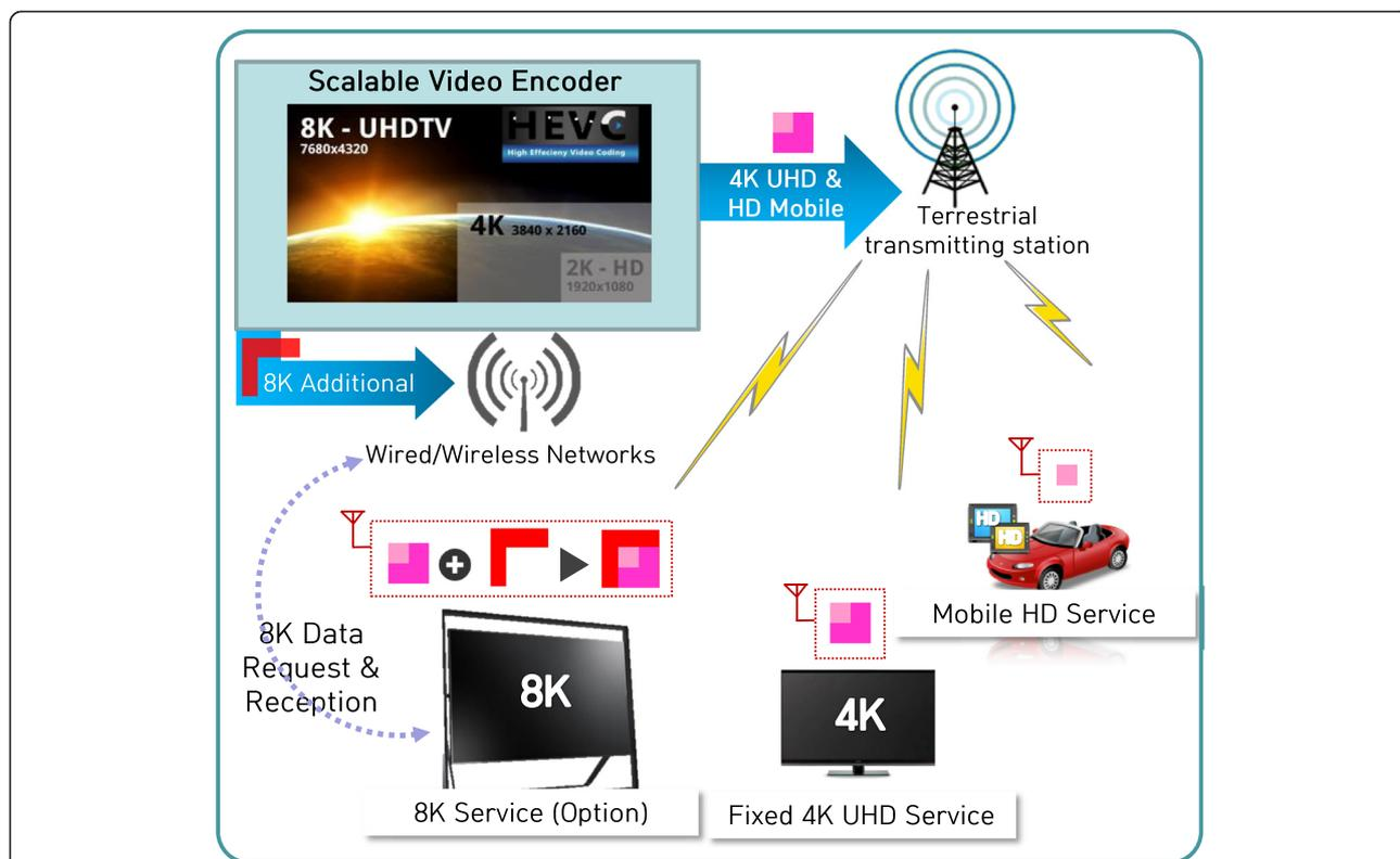
Figure 6 Concept diagram of terrestrial 4 K UHD and HD convergence broadcasting service through a single channel.
