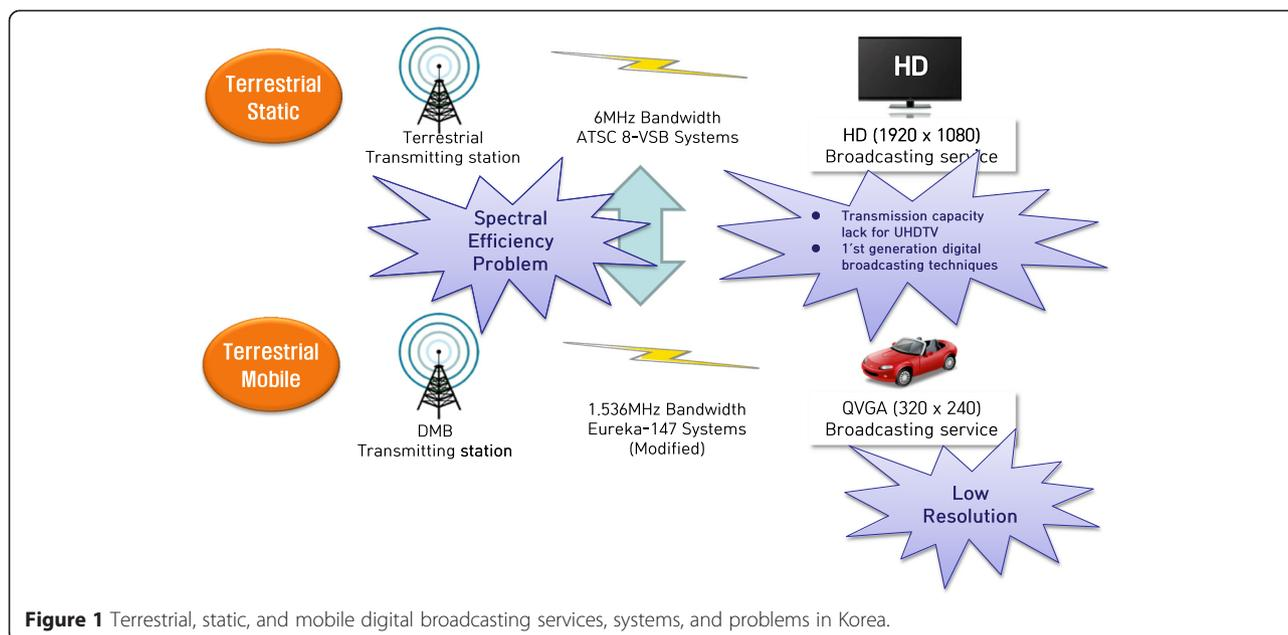
**Figure 1** Terrestrial, static, and mobile digital broadcasting services, systems, and problems in Korea.
