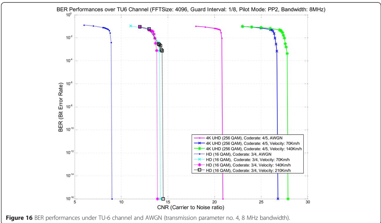
Figure 16 BER performances under TU-6 channel and AWGN (transmission parameter no. 4, 8 MHz bandwidth).
