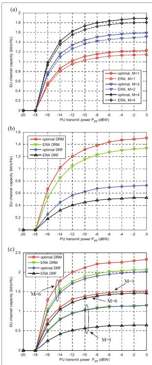
**Fig. 2** SU achievable rate versus PU transmit power  $P_{\rm PT}$  for **a** the cognitive OWT-RA network, **b** the cognitive TWT-DL network, and **c** the cognitive TWT-RA network
