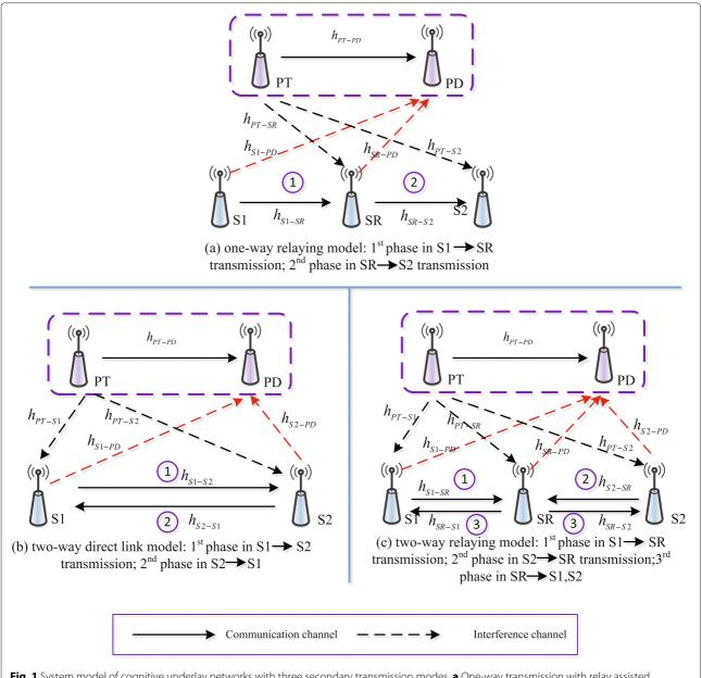
**Fig. 1** System model of cognitive underlay networks with three secondary transmission modes. **a** One-way transmission with relay assisted (OWT-RA), **b** two-way transmission with a direct link (TWT-DL), and **c** two-way transmission with relay assisted (TWT-RA)
