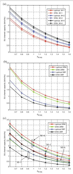
**Fig. 4** SU achievable rate versus PU parameter  $\sigma_{\rm PT-PD}^2$  for **a** the cognitive OWT-RA network, **b** the cognitive TWT-DL network, and **c** the cognitive TWT-RA network
