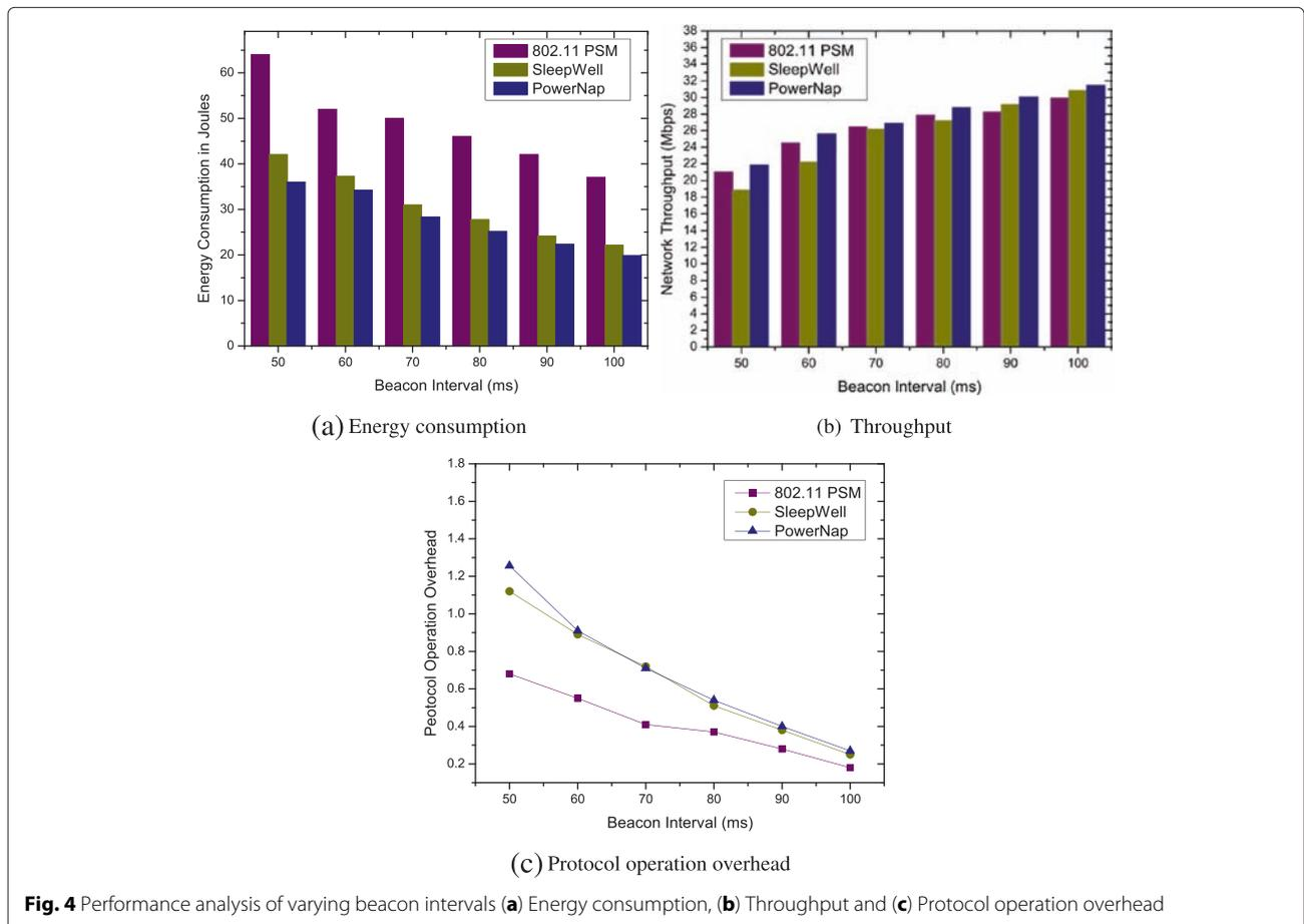
**Fig. 4** Performance analysis of varying beacon intervals (a) Energy consumption, (b) Throughput and (c) Protocol operation overhead
