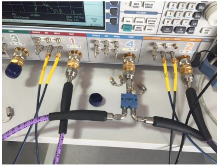
Fig. 2 Photo of cables connected to the VNA
