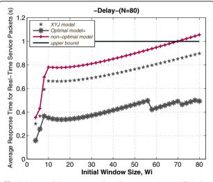
**Fig. 5** Average delay versus initial window contention size  $(CW_{min})$
