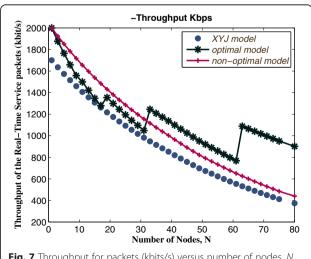
Fig. 7 Throughput for packets (kbits/s) versus number of nodes, N
