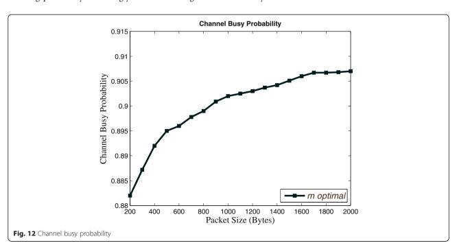
For 2000 bytes packets, the maximum performance is gained at the channel busy probability of 91 %.
