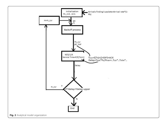
stage that MAC layer allows  $L_{\rm retry}$ . The default value of  $L_{\rm retry}$  in the IEEE 802.11 is 7. If the optimal number of backoff stages is larger than the default value, the m value will be set as  $L_{\rm retry}$ . Steps 22–25 search for the maximum m in each step, and Step 28 outputs the obtained result.
