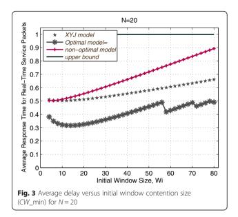
This indicates that the window size has a big impact on the average delay and our proposed scheme of adapting m and application rate can effectively maintain a stable and low transmission delay.
