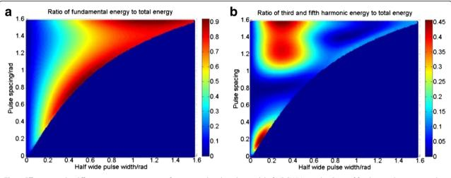
Fig. 6 Efficiency under different power consumptions for improved triple-pulse model of HP-PWM signal. a Ratio of fundamental wave to total energy. b The sum of the third and fifth harmonics to total energy
