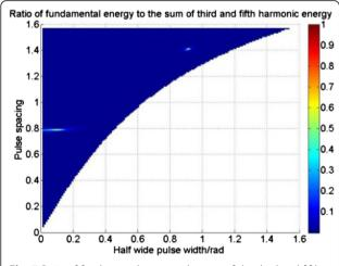
**Fig. 7** Ratio of fundamental wave to the sum of the third and fifth harmonics one
