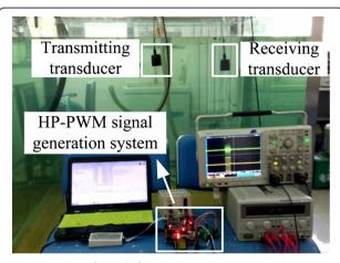
Fig. 8 Structure of test platform
