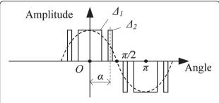
Fig. 4 Improved triple-pulse model of HP-PWM signal
