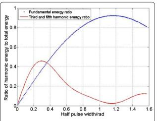
**Fig. 5** Efficiency under different conditions for single-pulse model of HP-PWM signal
