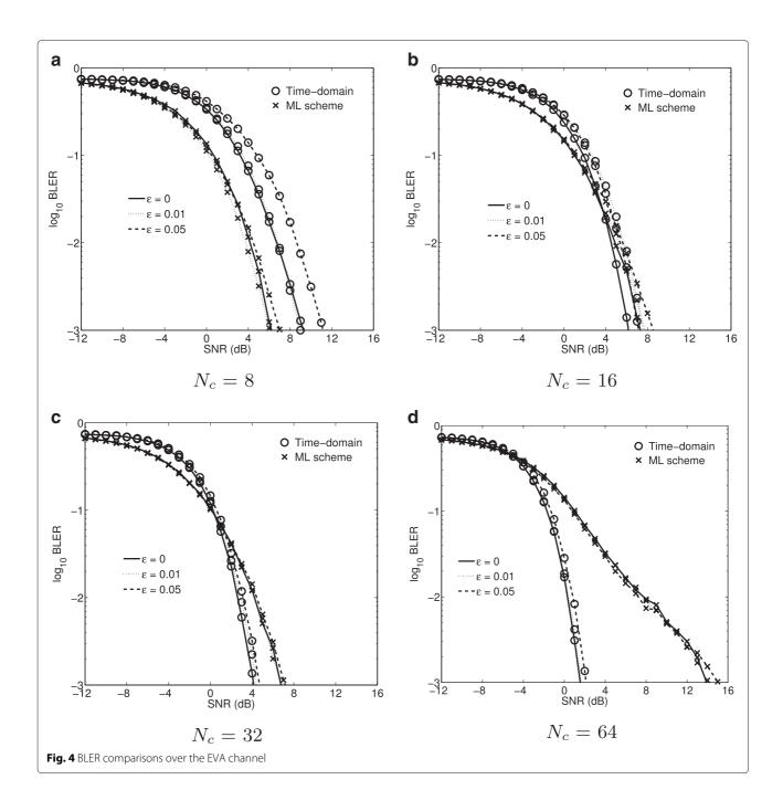
increased. This is because with increased  $N_c$ , more subcarriers may have experienced severe (deep) channel fading, which can lead to noise enhancement and hence poor detection.
