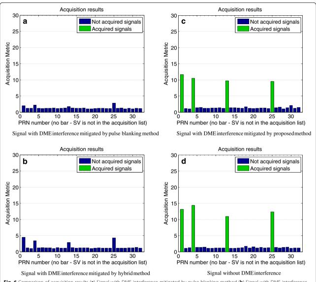
**Fig. 6** Comparison of acquisition results (**a**) Signal with DME interference mitigated by pulse blanking method (**b**) Signal with DME interference mitigated by hybrid method (**c**) Signal with DME interference mitigated by proposed method (**d**) Signal without DME interference
