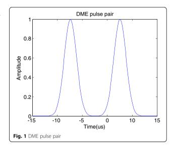
When the airborne DME equipment takes advantage of the 64–126 X channel for communication, the ground equipment may respond frequencies ranged from 1151 to 1213 MHz. Unfortunately, this frequency band covers the GPS L5 signal with central frequency 1176.45 MHz and bandwidth 24 MHz.
