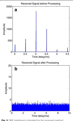
**Fig. 5** DME interference mitigated by the proposed method (a) Received signal before processing (b) Received signal after processing
