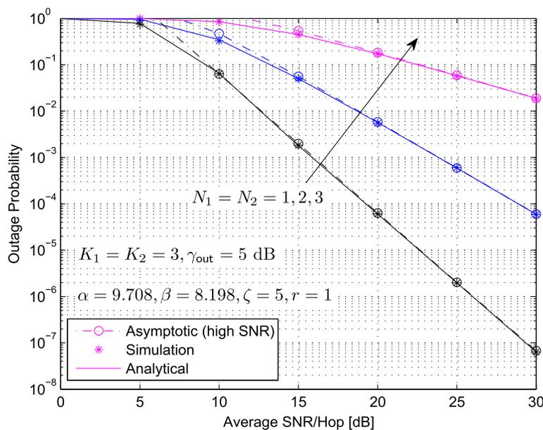
**Fig. 2**  $P_{\text{out}}$  vs SNR of multiuser mixed RF/FSO/RF relay network with generalized order user scheduling for different values of  $N_1 = N_2$
