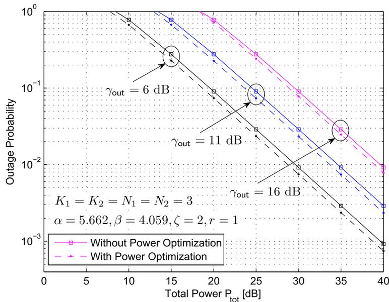
**Fig. 6**  $P_{out}$  vs SNR of multiuser mixed RF/FSO/RF relay network with generalized order user scheduling for different values of  $\gamma_{out}$  without and with power optimization
