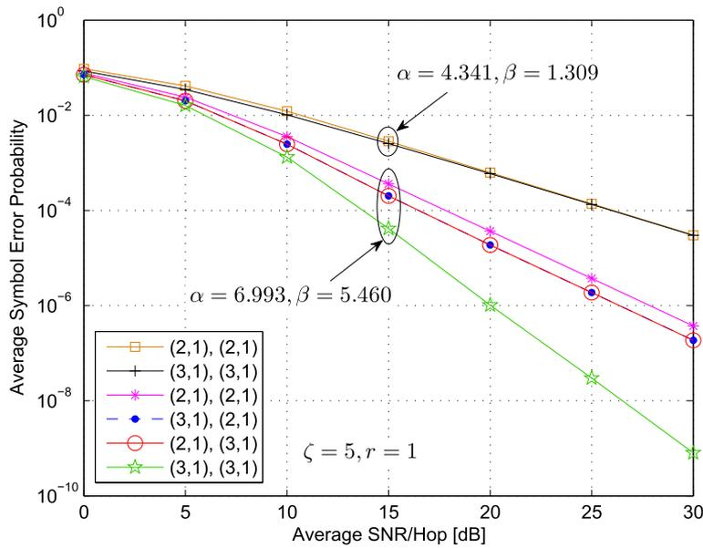
**Fig. 9** ASEP vs SNR of multiuser mixed RF/FSO/RF relay network with generalized order user scheduling for different values of  $(K_1, N_1)$ , and  $(K_2, N_2)$
