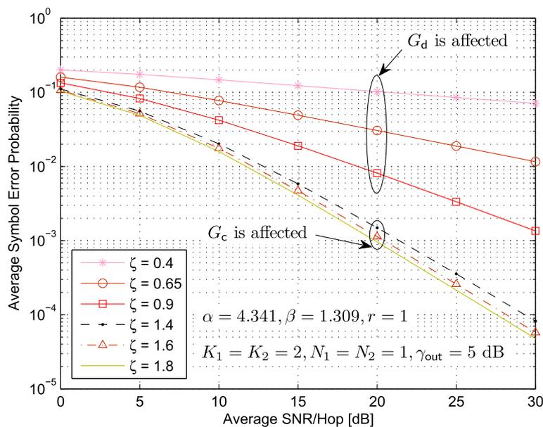
**Fig. 7** ASEP vs SNR of multiuser mixed RF/FSO/RF relay network with generalized order user scheduling for different values of  $\zeta$
