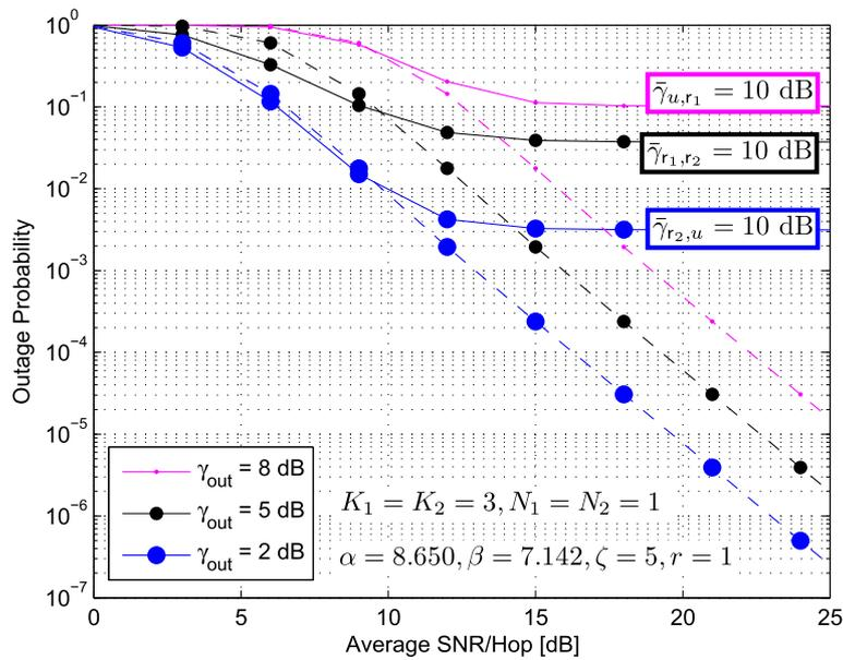
**Fig. 4**  $P_{out}$  vs SNR of multiuser mixed RF/FSO/RF relay network with generalized order user scheduling for different values of  $\gamma_{out}$  with fixed average SNRs and varying average SNRs
