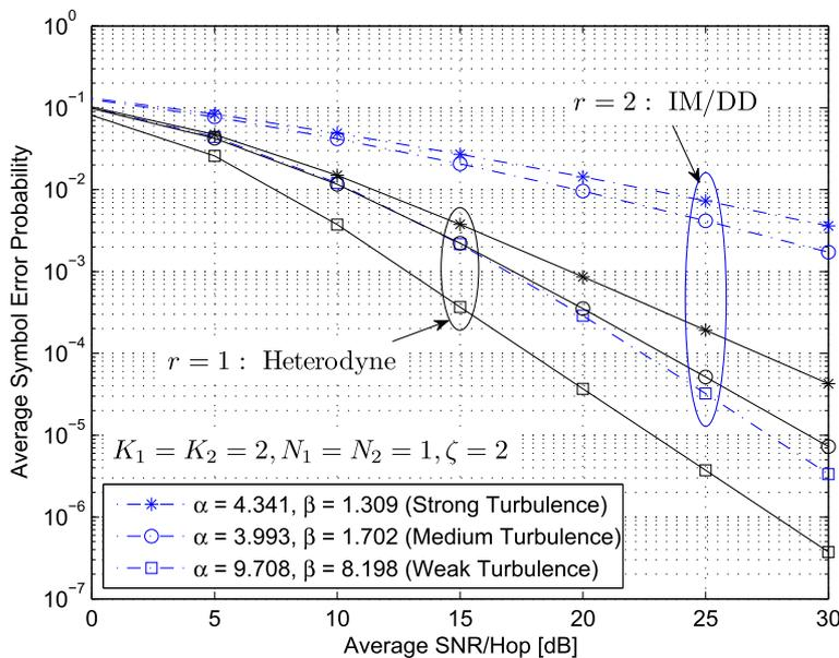
**Fig. 8** ASEP vs SNR of multiuser mixed RF/FSO/RF relay network with generalized order user scheduling for different values of  $\alpha$ ,  $\beta$ , and  $r$
