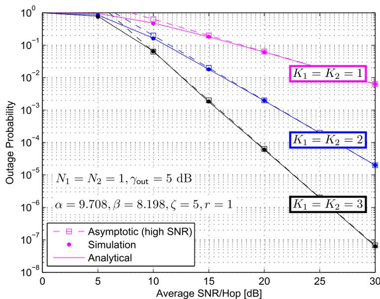
**Fig. 3**  $P_{out}$  vs SNR of multiuser mixed RF/FSO/RF relay network with generalized order user scheduling for different values of  $K_1 = K_2$
