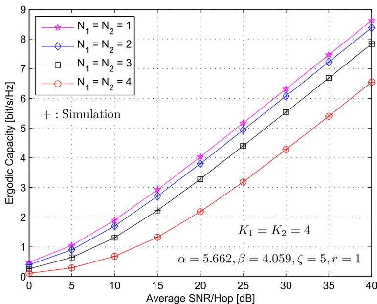
**Fig. 10** Capacity vs SNR of multiuser mixed RF/FSO/RF relay network with generalized order user scheduling for different values of  $N_1 = N_2$
