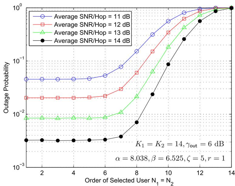
**Fig. 5**  $P_{out}$  vs order of selected user of multiuser mixed RF/FSO/FSO relay network with generalized order user scheduling for different values of average SNR
