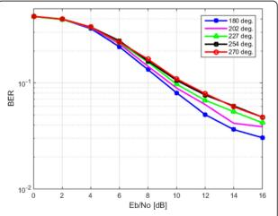
Fig. 8 Performance degradation due to changing channel fading for random body direction in quadrant III
