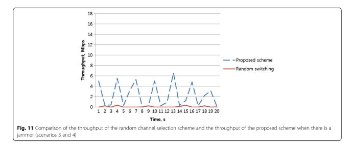
described in subsection 3.1. If we compare Figs. 10 and 11, the throughput is lower for Fig. 11 because of the interference from the jammer.
