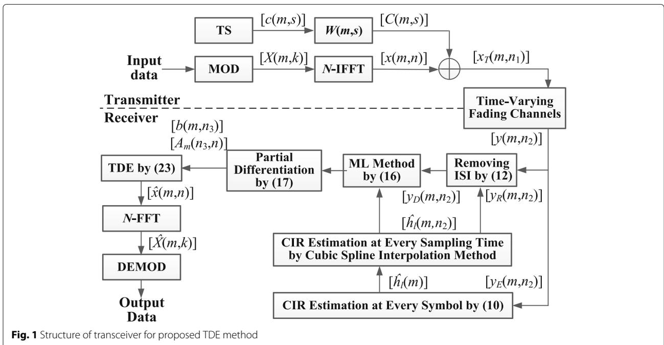
Fig. 1 Structure of transceiver for proposed TDE method
