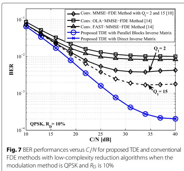
Fig. 7 BER performances versus C/N for proposed TDE and conventional FDE methods with low-complexity reduction algorithms when the modulation method is QPSK and  $R_D$  is 10%
