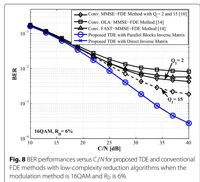
Fig. 8 BER performances versus C/N for proposed TDE and conventional FDE methods with low-complexity reduction algorithms when the modulation method is 16QAM and  $R_D$  is 6%
