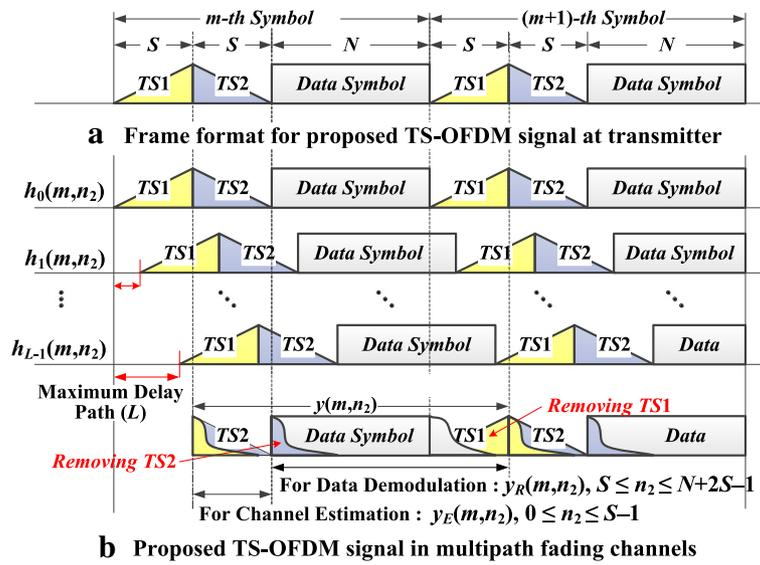
**Fig. 2** Structure of frame format for TS-OFDM signal at transmitter and receiver. **a** Frame format for proposed TS-OFDM signal at transmitter. **b** Proposed TS-OFDM signal in multipath fading channels
