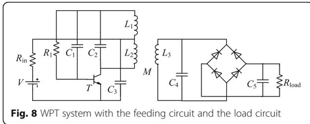
**Fig. 8** WPT system with the feeding circuit and the load circuit
