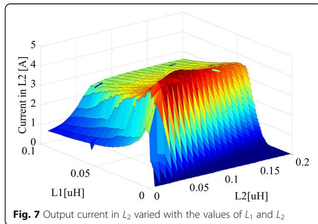
Fig. 7 Output current in  $L_2$  varied with the values of  $L_1$  and  $L_2$
