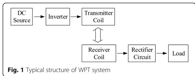
source, inverter, transmitter, receiver, rectifier circuit, and load. The inverter is applied to invert the DC source into a sinusoidal source to provide a shifting current in the transmitter coil. In the previous research, the works about the WPT system almost focus on the coil design when the system is optimized [10–12]. In the system, the inverter circuit is too complicated to be optimized along with the coil system.
