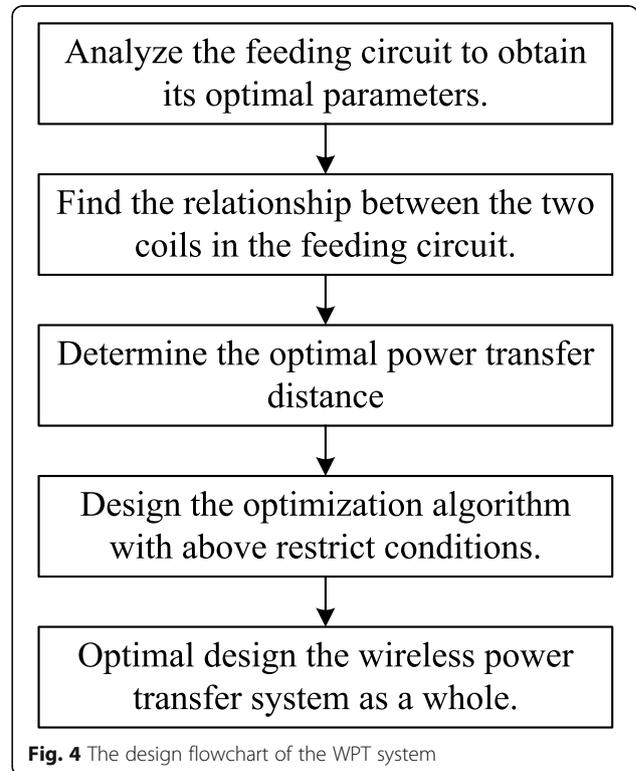
**Fig. 4** The design flowchart of the WPT system
