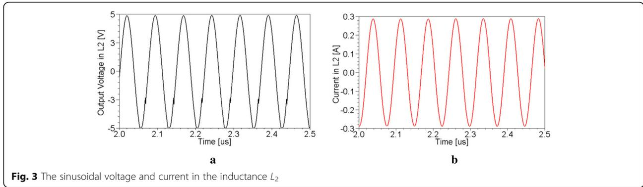
**Fig. 3** The sinusoidal voltage and current in the inductance  $L_2$
