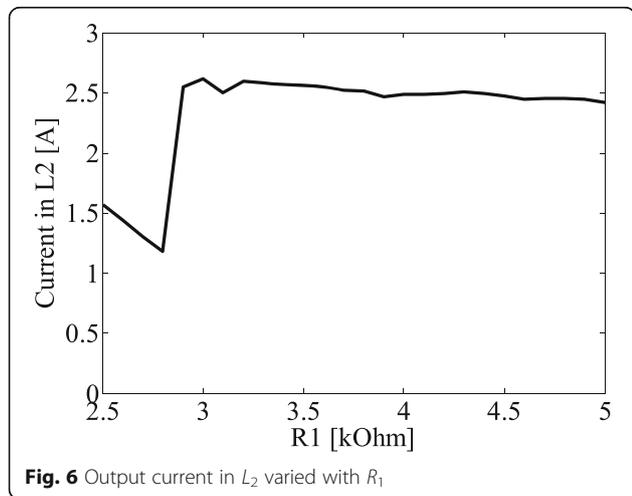
Fig. 6 Output current in  $L_2$  varied with  $R_1$
