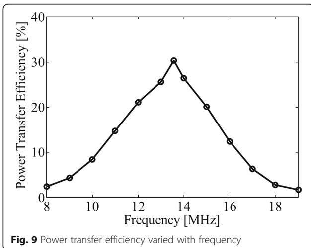
**Fig. 9** Power transfer efficiency varied with frequency
