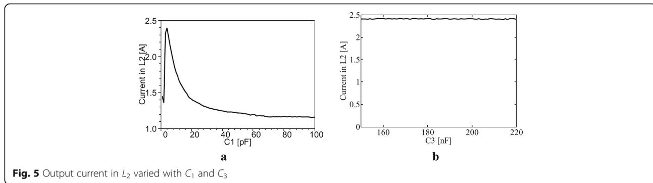
Fig. 5 Output current in  $L_2$  varied with  $C_1$  and  $C_3$
