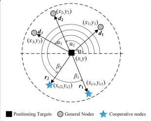
Fig. 2 Geometry of the nodes in two-dimensional cooperative localization scenario
