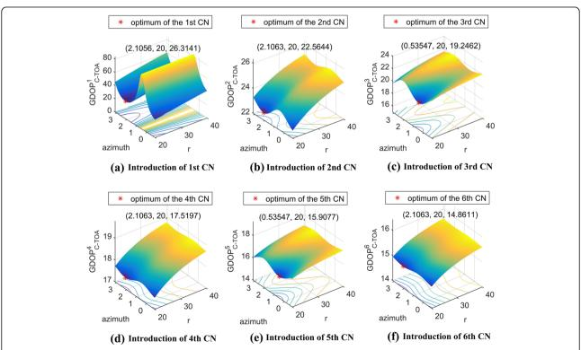
Fig. 5 Performance of partial exhaustive method towards AOA-based system in environment 1. a Introduction of the first CN. b Introduction of the second CN. c Introduction of the third CN. d Introduction of the fourth CN. e Introduction of fifth CN. f Introduction of sixth CN
