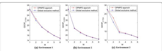
Fig. 9 Accuracy comparison of OPMPD approach and global exclusive method towards AOA-based system. a Environment 1. b Environment 2. c Environment 3
