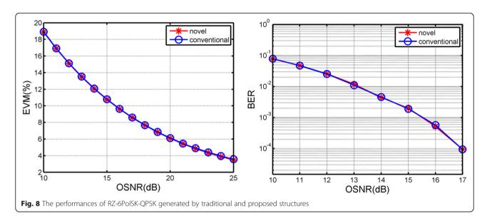
Figure 6 shows the EVM and BER results with different OSNR (0.1 nm); the results of traditional and proposed are shown together as comparisons. As shown in Fig. 6, the EVM decreased as the OSNR increased, the EVM is less than 10% when OSNR >18 dB, and the BER is below  $10^{-3}$  when OSNR >18 dB. The results show the performance of the two transmitters are nearly the same; the proposed structure even has a little better performance.
