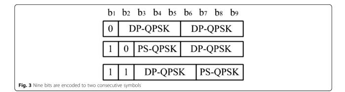
In order to get the four basic phase shift, the driven signals should have four different levels to form the points in DP-QPSK or PS-QPSK. With the coding rules, we can get the 6PolSK-QPSK at the output.
