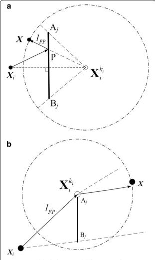
**Fig. 1** TOA model of reflection and diffraction. **a** Reflection. **b** Diffraction
