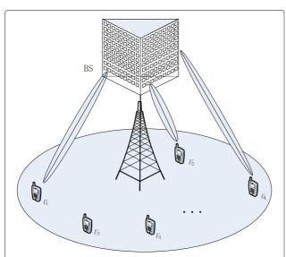
**Fig. 1** A schematic diagram of the multi-user MIMO mmWave system, where a BS equipped with a URA serves *K* users
