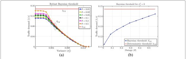
**Fig. 11** Example of on/off switching robust Bayesian threshold for different values of outage probability  $\theta$  and variance  $\sigma_p^2$ . For comparison purposes, the deterministic threshold  $\lambda_{TH}$  is also depicted. **a** Bayesian threshold as a function of the variance  $\sigma_p^2$  for different outages. **b** Bayesian threshold as a function of the outage probability for  $\sigma_p^2 = 0$
