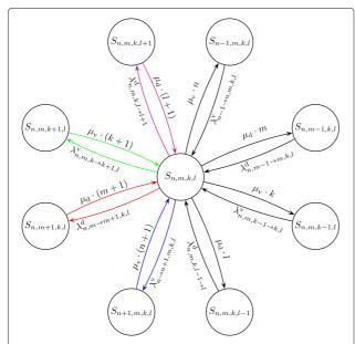
Fig. 4 Examples of the allowed states of the 4D M/M/m/m Markov chain
