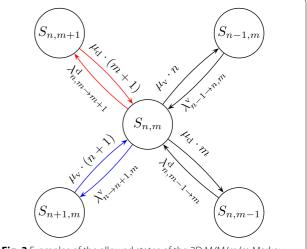
Fig. 3 Examples of the allowed states of the 2D M/M/m/m Markov chain
