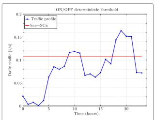
**Fig. 8** On/off switching threshold example for a single traffic profile during the first year with traffic type TP1
