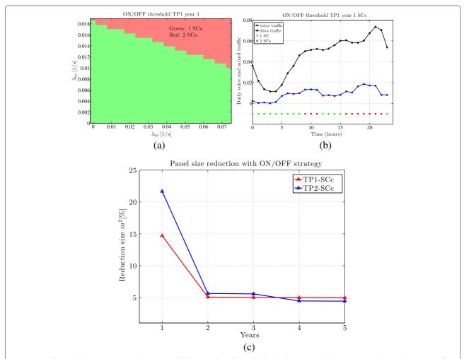
Fig. 10 On/off threshold region, hours to be switched off for a specific traffic profile for the first year, and solar panel size reduction for mixed traffic. a Region of lambda threshold for mixed traffic be On/off threshold example for mixed traffic profile. c Solar panel size reduction for mixed traffic and two different traffic profiles
