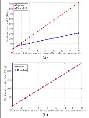
**Fig. 7** Backhaul bitrates for voice and data connections. **a** Backhaul bitrates according to the number of voice connections. **b** Backhaul bitrates according to the number of data connections
