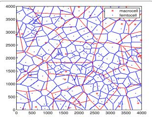
**Fig. 2** The network is modeled as a superposition of two independent Voronoi tessellations
