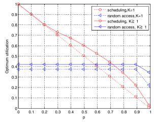
**Fig. 8** Optimum utilization for MSS under scheduling-based and random access schemes
