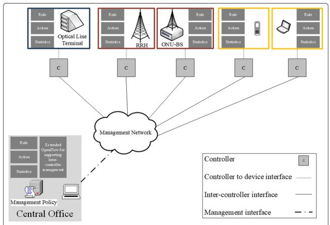
Fig. 8 An SDN controller management network. A management policy is applied to the SDN network through a management computer located at the CO
