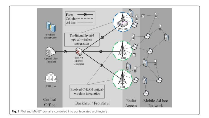
domain depends on the location where the backhaul data are decoded, so it is technology-specific. At the edge of the network, mobile nodes form a multi-hop spontaneous network (denoted as MANET) that can be regarded as an independent domain, locally able to dispatch packets without exploiting the cellular infrastructure.
