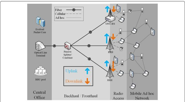
Fig. 6 Traffic engineering paradigm by adjusting the uplink-to-downlink ratio in the fronthaul network to support traffic engineering in the MANET domain
