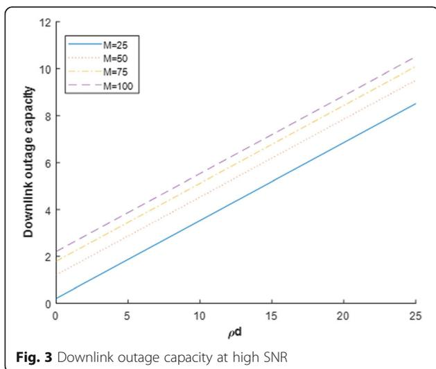
Fig. 3 Downlink outage capacity at high SNR
