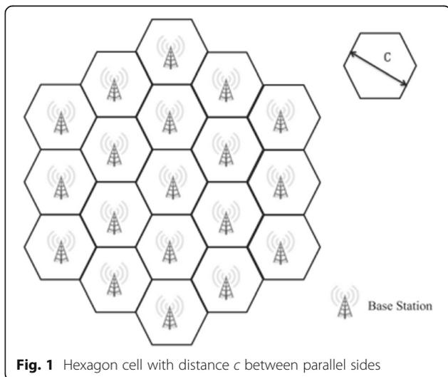
Fig. 1 Hexagon cell with distance  $c$  between parallel sides
