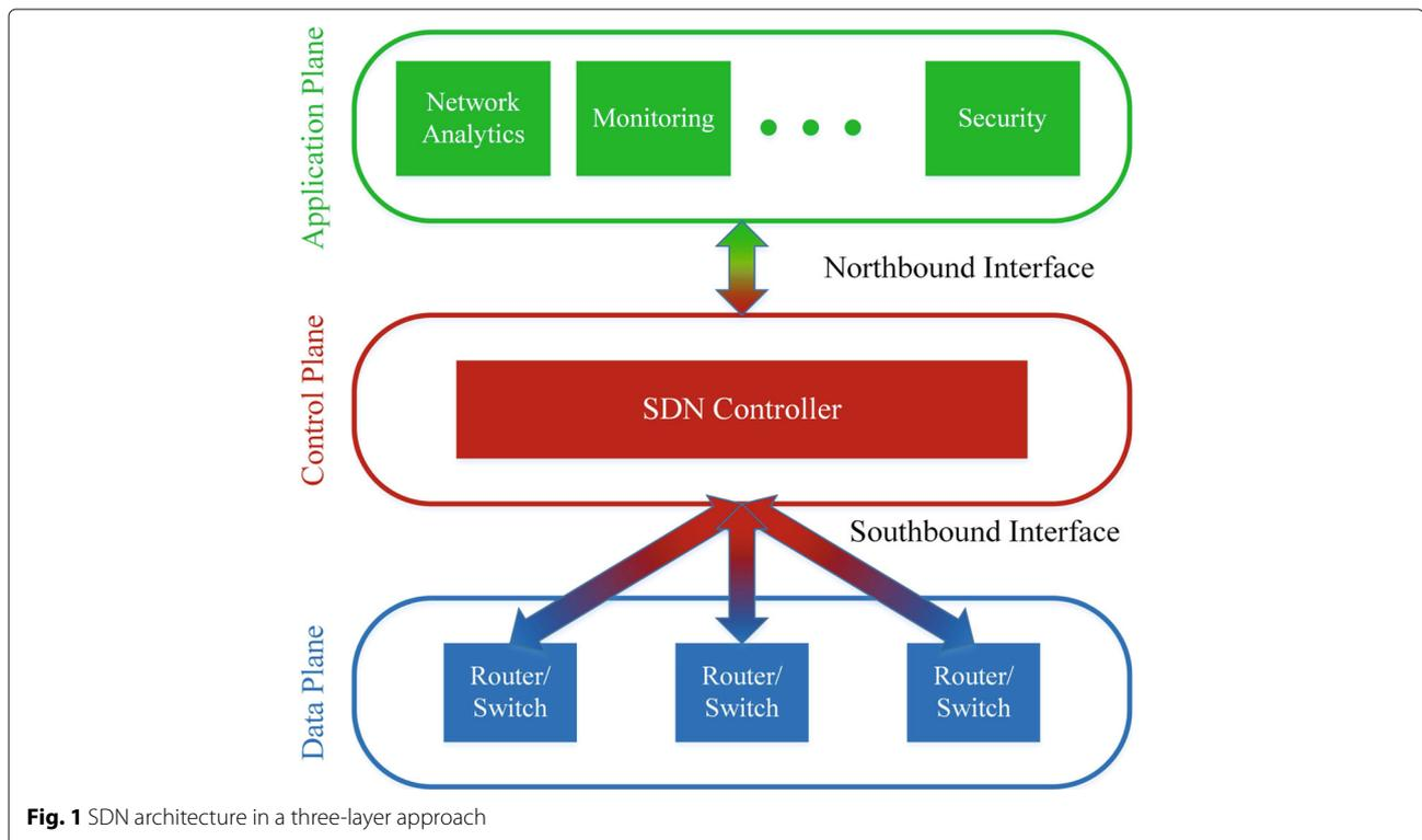
**Fig. 1** SDN architecture in a three-layer approach
