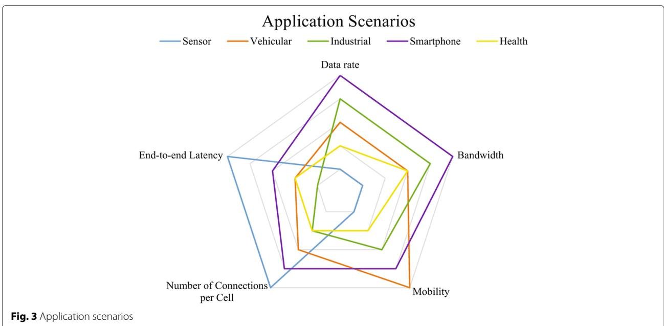
Figure 3 highlights the necessity of incorporating network slicing, as virtual networks tailored to specific requirements have better performance than typical multipurpose networks. Moreover, a network slice can be modified, depending on service requirements and number of users. Slices are also isolated to each other, which enhances reliability and security, as configurations of different slices do not affect each other.
