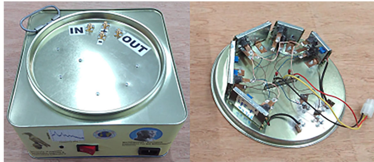
Fig. 8 Electromagnetic shielding metallic box. Apart from the preamplifier stage, the amplification and filtering stages (second to sixth) are all arranged inside a metallic box for electromagnetic shielding purposes. The total PCB circuits are mechanically adapted at the inner side of the box top. That arrangement allows us to adjust the total voltage gain through applying torque to the potentiometer screw at the variable gain amplifier. A connector at the outer side of the metallic box provides power supply at the amplification and filtering stages through an outer switch
