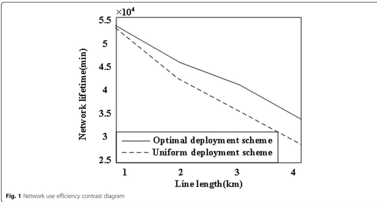
network life cycle and use efficiency of the optimized deployment strategy are better than the equal distance deployment strategy. The life cycle of these two deployment strategies decreases with the increase of network length, but the reduction degree of network life cycle of the optimized deployment strategy is less. When the monitoring length is 4000 m, the network life cycle of the optimized deployment strategy is 20% higher than
