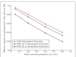
**Fig. 5** Effective capacity versus delay constraint,  $\theta_0$  in a heterogeneous 3-hop AF relay network;  $B_0 = 10^{-5}$ ,  $\bar{s_0} = 2$  dB,  $m_0 = 1$ ,  $\bar{P_0} = 1$  W/Hz;  $\bar{s_1} = 3$  dB,  $m_1 = 1$ ,  $\bar{P_1} = 1.5$  W/Hz;  $\bar{s_2} = 4$  dB,  $m_2 = 2$ ,  $\bar{P_2} = 1$  W/Hz
