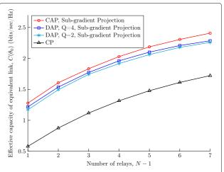
**Fig. 3** Effective capacity versus number of relays, when path length is constant, path loss exponent  $\zeta = 3$ , total average power consumption is fixed to 3 W/Hz,  $B_0 = 10^{-5}$ ,  $\theta_0 = 0.1$  and Nakagami-m fading channels with  $m_i = 2$ ,  $0 \le i \le N - 1$
