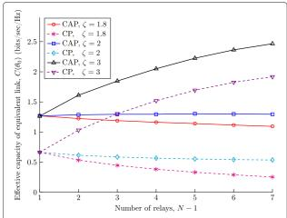
**Fig. 4** Effect of increasing the number of relays, when the length of line of sight path is fixed and total transmission power is fixed for different path loss exponents,  $\sum_{i=0}^{N-1} \bar{P}_i = 3$  W/Hz,  $\theta_0 = 0.1$
