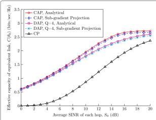
**Fig. 2** Effective capacity versus average SINR of each hop in different power adaptation schemes, when parameters are obtained analytically or by sub-gradient projection, Rayleigh fading channels  $S_0 = E\{s_i\}$ ,  $\bar{P}_i = 1$  W/Hz,  $0 \le i \le 2$ ,  $B_0 = 10^{-5}$ ,  $\theta_0 = 0.05$
