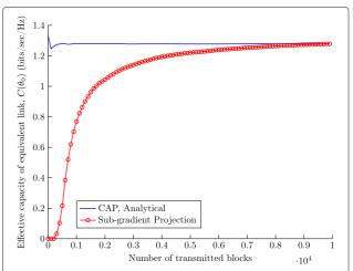
**Fig. 6** Effective capacity versus number of transmitted blocks; analytical approach compared with the sub-gradient projection method;  $E\{s_i\}=10$  dB,  $\bar{P}_i=1$  W/Hz,  $0 \le i \le 2$ ,  $B_0=10^{-5}$ ,  $\theta_0=0.01$ , and Nakagami-m fading channels with  $m_i=3$ ,  $0 \le i \le 2$
