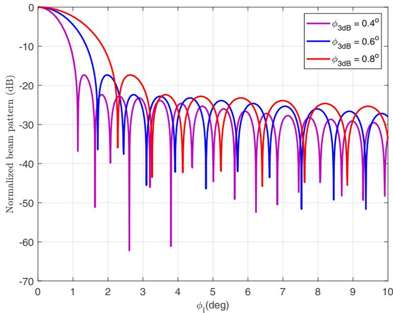
**Fig. 2** Normalized beam pattern with different 3 dB angles. This figure presents normalized beam pattern when the 3 dB angles are 0.4°, 0.6°, and 0.8°, respectively
