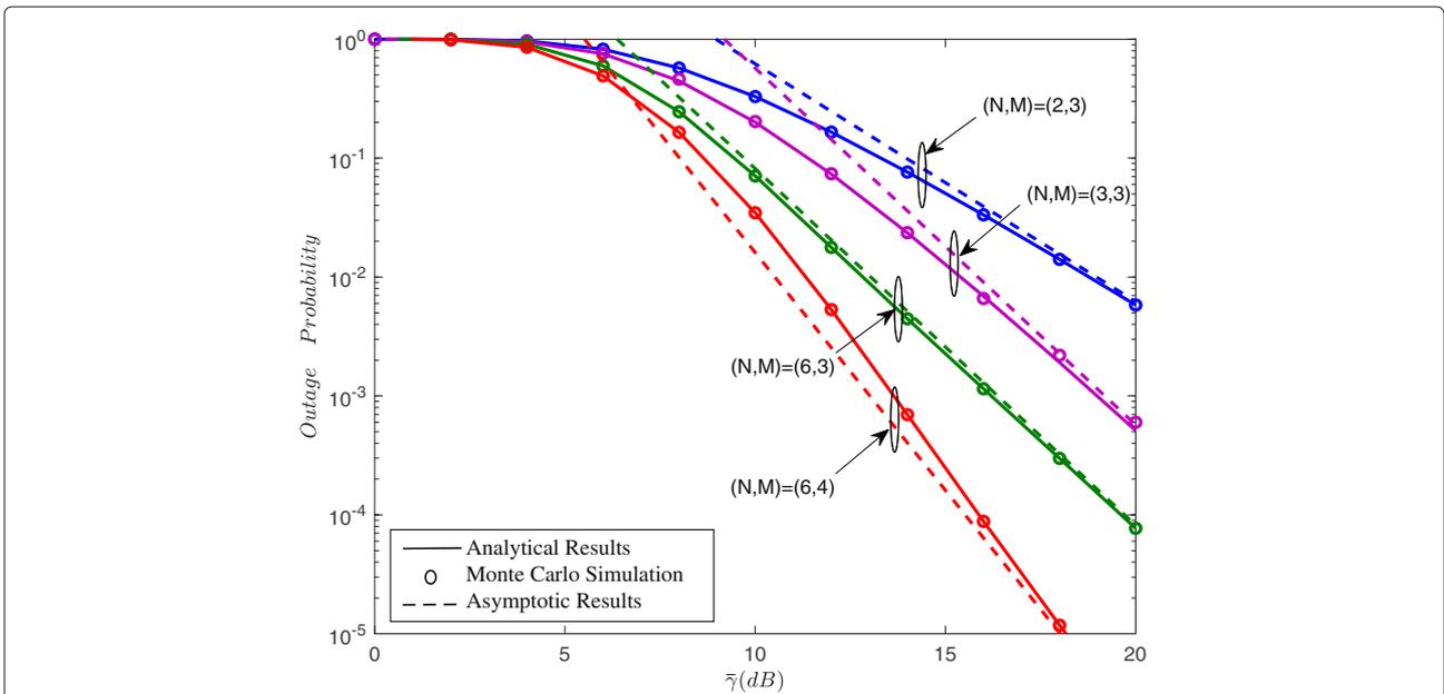
**Fig. 4** Analytical and asymptotic OP with OS/MRC scheme. This figure gives the exact and asymptotic OP versus  $\bar{\gamma}$  with OS/MRC scheme when both uplink and downlink undergo FHS fading. In addition, Monte Carlo simulations verify their correctness
