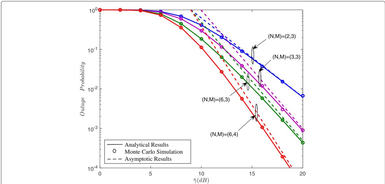
**Fig. 3** Analytical and asymptotic OP with OS/SC scheme. This figure gives the exact and asymptotic OP versus  $\bar{\gamma}$  with OS/SC scheme when both uplink and downlink undergo FHS fading. In addition, Monte Carlo simulations verify their correctness
