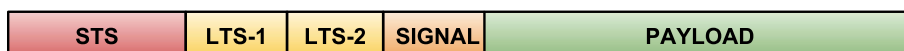
Fig. 3 WiFi frame structure: LTS-1 and LTS-2 are used for channel and noise variance estimation
