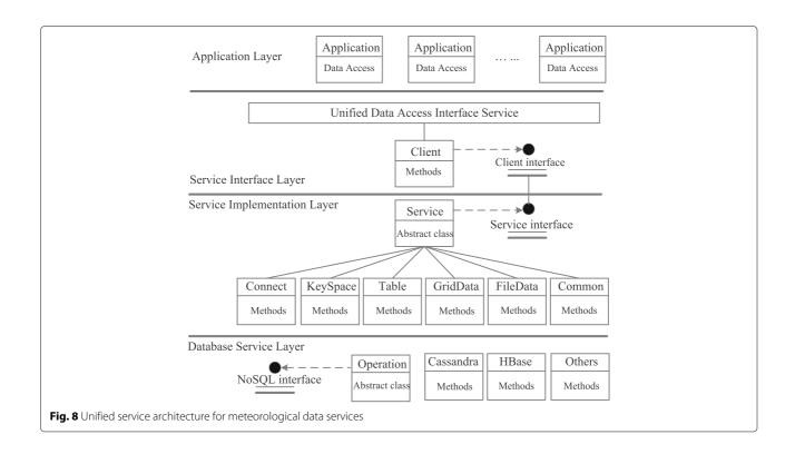
interface services. Applications can access meteorological data by RESTful Interface, Web Service Interface, and distributed Client SDK, which uses meteorological data algorithm as component or service of application program.
