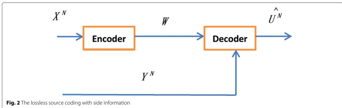
**Fig. 2** The lossless source coding with side information
