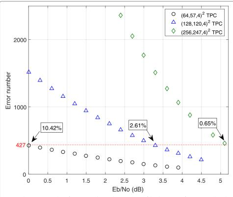
**Fig. 10** The average number of errors according to the SNR region of the three types of TPCs received via the AWGN channel
