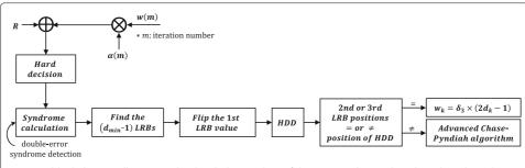
**Fig. 3** A block diagram illustrating the detailed procedure of the proposed HISO decoding algorithm when detecting the double-error syndrome
