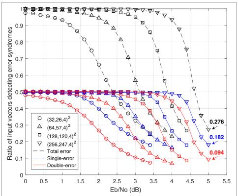
**Fig. 2** Ratios of input vectors detecting error syndromes (black: total error, blue: single-error, red: double-error) according to the SNR increment during the TPC decoding based on the Chase-Pyndiah algorithm. We assumed that both the number of maximum iteration and LRBs as 4
