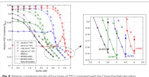
**Fig. 9** Relative complexity results of four types of TPCs compared with the Chase-Pyndiah decoding algorithm [2] in terms of HDD requirements. ( $l_{max}$ , 8; LRB number, 4)
