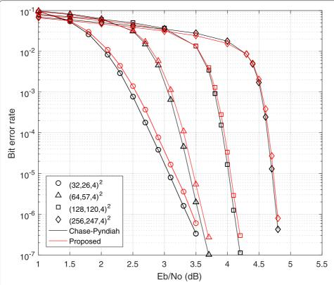
**Fig. 12** Error correction performance results of the Chase-Pyndiah and the proposed decoding algorithm in three kind of TPCs ( $I_{max}$ , 8; LRB number, 4.)
