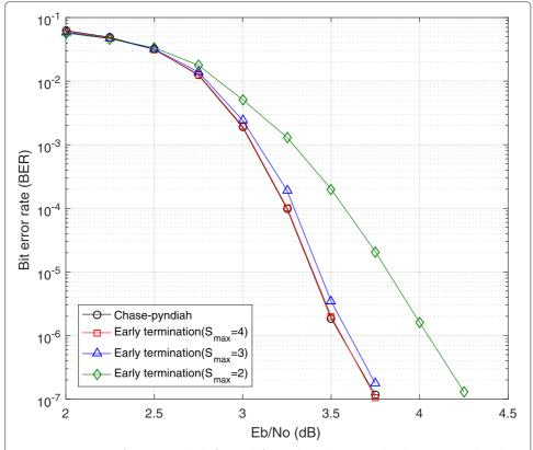
**Fig. 7** Bit error rate performance results before and after applying the proposed early termination algorithm to  $(64, 57, 4)^2$  TPC.  $I_{max}$ , 8 (i.e., the number of maximum full-iterations, 4), LRB number, 4
