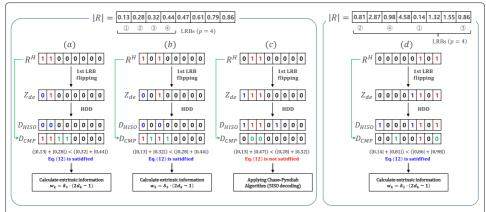
**Fig. 4** Examples performing the proposed HISO decoding algorithm when containing two errors in the input vector. Example (a) and (b) represent the cases of successful error correction via the proposed HISO decoding. By contrast, example (c) illustrates the case of wrong error correction. Example (d) shows the valid codeword is generated, but it is not the correct codeword
