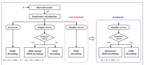
**Fig. 1** A block diagram illustrating the main concept of the proposed syndrome-based decoding algorithm. The red box represents the conventional decoding technique (SISO decoding) when the double-error syndrome is detected, and we want to modify it like the blue box (a combination of advanced HISO and SISO decoding)
