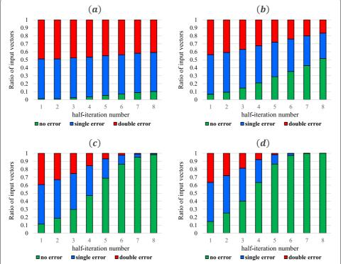
**Fig. 5** Ratios of input vectors detecting each syndrome (green: no-error, blue: single-error, red: double-error) in the  $(64, 57, 4)^2$  TPC according to the SNR regions when error correction is performed based on the Chase-Pyndiah algorithm. **a** SNR 1.0 dB corresponding to BER  $10^{-1}$ . **b** SNR 2.75 dB corresponding to BER  $10^{-2}$ . **c** SNR 3.25 dB corresponding to BER  $10^{-4}$ . **d** SNR 3.5 dB corresponding to BER  $10^{-6}$
