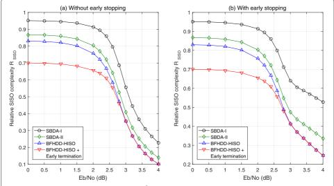
**Fig. 8** Relative complexity results for (64,57,4)<sup>2</sup> TPC compared to the Chase-Pyndiah decoding algorithm [2] in terms of the SISO decoding requirements. **a** Without early stopping. **b** With early stopping. ( $l_{max}$ , 8; LRB number, 4)
