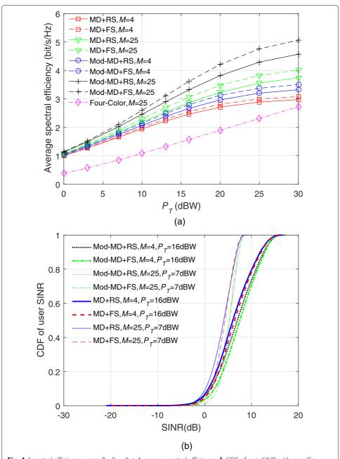
**Fig. 4** Spectral efficiency verse  $P_T$ , R=2. **a** Average spectral efficiency. **b** CDF of user SINR with specific parameters
