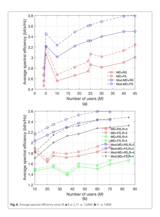
scenario shows an almost linear growth. The results indicate that the system with four-color frequency reuse is power-limited, and system with full-frequency reuse scenario is interference-limited.
