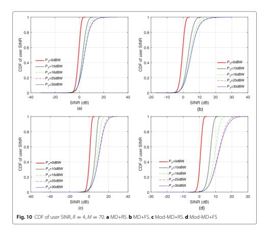
declines with the increase in  $P_T$ , owing largely to the interference-limited characteristics of the system.
