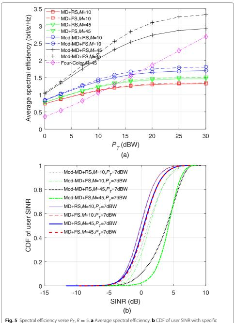
**Fig. 5** Spectral efficiency verse  $P_T$ , R=5. **a** Average spectral efficiency. **b** CDF of user SINR with specific parameters,  $P_T=7dBW$
