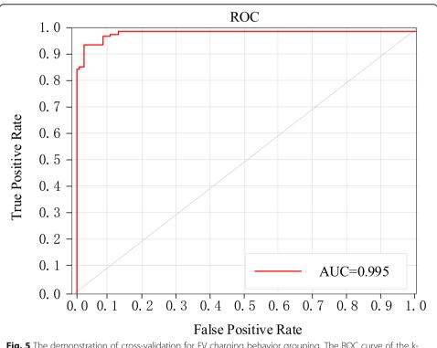
**Fig. 5** The demonstration of cross-validation for EV charging behavior grouping. The ROC curve of the knearest neighbor (KNN)-based EV charging behavior classification algorithm is shown in this figure
