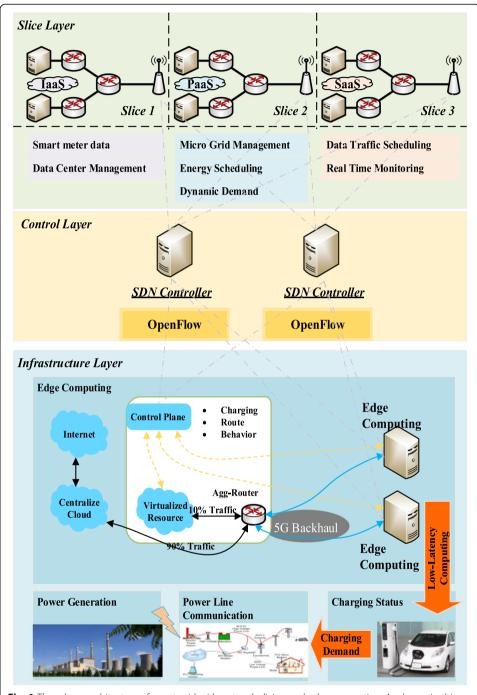
**Fig. 1** Three-layer architecture of smart grid with network slicing and edge computing. As shown in this figure, it provides a smart grid network architecture based on network slicing and edge computing to abstract or share substrate resources
