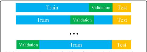
**Fig. 4** The demonstration of cross-validation for EV charging behavior grouping. As shown in this figure, there are 223 user data after filtering; we divided them into 6 groups. The first 5 groups are used for cross-validation, and the last group is used for final validation
