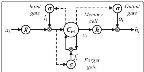
**Fig. 3** The structure of the LSTM predictor. This figure illustrates the typical architecture of LSTM predictor. A representative LSTM neural network cell mainly contains four gates with different functions including the input gate, the input modulation gate, the forget gate, and the output gate
