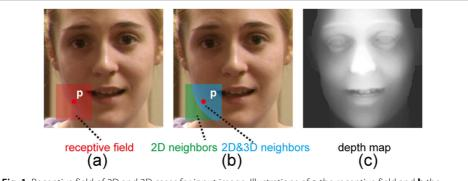
**Fig. 1** Receptive field of 2D and 3D cases for input image. Illustrations of **a** the receptive field and **b** the difference of 2D and 3D neighbors for a given pixel p, and **c** the corresponding depth map
