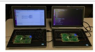
Fig. 3 The USRP B210 used in the experiments
