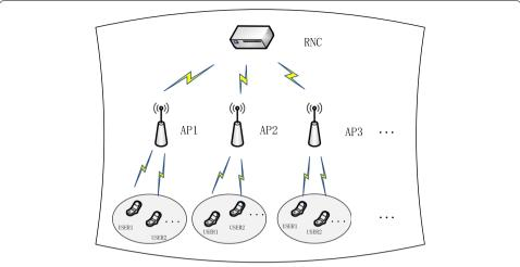
**Fig. 1** System model based on game theory. A three-layer heterogeneous fusion network model is composed of RNC, base stations and base station users
