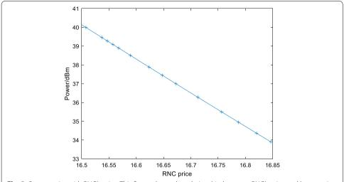
**Fig. 3** Power varies with RNC's price. This figure shows the relationship between RNC's price and base station power
