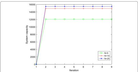
**Fig. 6** Comparison of system capacity. We set the number of base stations to 5, 15 and 25, respectively. With the increase in the number of base stations, the total capacity of the system based on the proposed power allocation algorithm will increase
