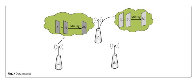
Node i keeps slice  $X_i$  and sends slice  $Y_i$  to one of its neighboring node in order to hide the raw data. Figure 6 demonstrates the process of slicing based on the extended Euclidean decomposition.
