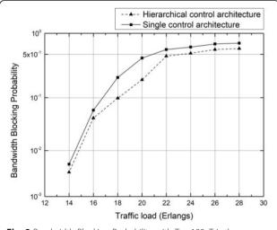
Fig. 8 Bandwidth Blocking Probability with T = 100. T is the threshold of spectrum fragmentation degree
