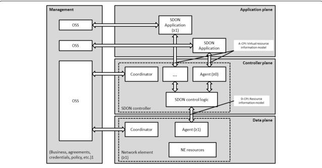
Fig. 1 The hierarchical structure of SDON. This architecture includes four planes: data plane, controller plane, application plane and management plane
