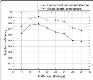
Fig. 9 Spectrum efficiency with  $T=100.\,T$  is the threshold of spectrum fragmentation degree
