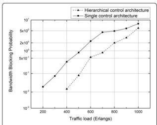
**Fig. 4** The Bandwidth Blocking Probability under two architectures. The solid line and dotted line represent the bandwidth blocking probability of hierarchical control architecture and single control architecture, respectively
