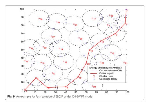
the hop number is 10. This illustrates that the algorithm combining SWIPT and routing may find a more energy-efficient transmission path.
