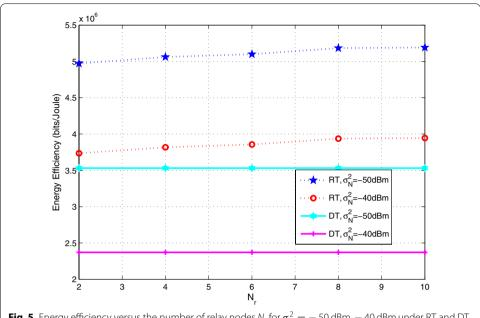
**Fig. 5** Energy efficiency versus the number of relay nodes  $N_{\rm f}$  for  $\sigma_{\rm fj}^2=-$  50 dBm, - 40 dBm under RT and DT modes
