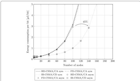
**Fig. 11** Saturated scenarios (1&2): The average energy consumption with no interference in saturated traffic conditions shows that IB-CSMA/CD is more energy efficient if more than 20 nodes are in the network compared to HD-CSMA/CA and FD-CSMA/CA
