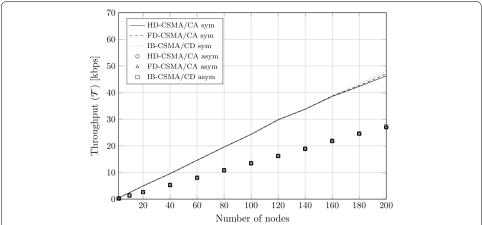
**Fig. 10** Unsaturated scenarios (3 and 4): The throughput in unsaturated traffic conditions increases linearly in all schemes. There is no difference in throughput between the different schemes
