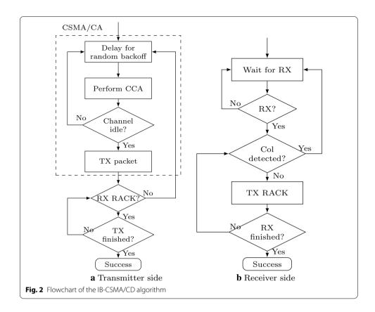
is transmitted in the uplink and collisions or interference are simultaneously detected in the downlink. Our earlier work [15, 17] proposed the IB-CSMA/CD scheme to leverage this information to optimize throughput, delay and energy.
