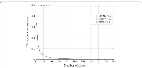
**Fig. 9** The AP fairness in symmetric traffic conditions shows that FD-CSMA/CA achieves a fair 0.5 downlink/uplink ratio in all situations while the other two schemes follow a 1/N curve
