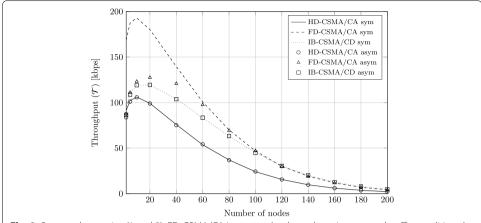
Fig. 8 Saturated scenarios (1 and 2): FD-CSMA/CA increases the throughput in saturated traffic conditions by 2 compared to HD-CSMA/CA. The increase of IB-CSMA/CD compared to HD-CSMA/CA is between 1.2 and 2
