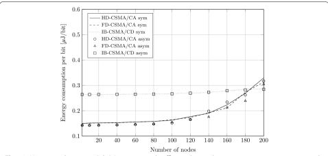
**Fig. 12** Unsaturated scenarios (3&4): In unsaturated traffic conditions, the average energy consumption with no interference shows only a minor difference between the three cases
