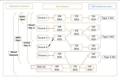
**Fig. 4** NSI configuration types for micro-operator deployment scenarios [4, 31]. This figure show the mapping of different NSI configuration types for each deployment scenario of a micro-operator
