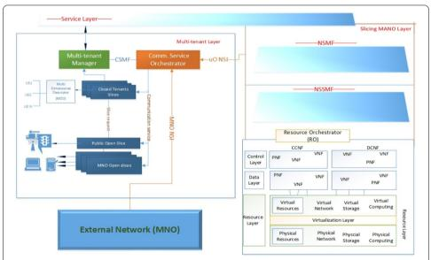
**Fig. 9** Micro-operator slicing architecture with focus on the multi-tenant layer [11]. The figure present an extended version of the micro-operator slicing architecture based on Fig. 6 with focus on the multi-tenant layer
