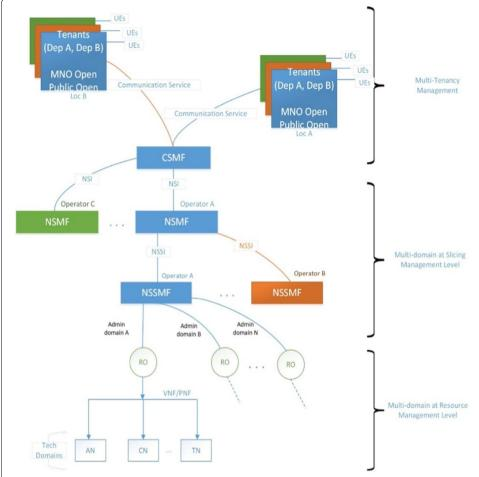
**Fig. 5** Simplified description of multi-domain using 3GPP functionalities. This figure presents a description of achieving multi-tenancy and multi-domain and their importance in network virtualization
