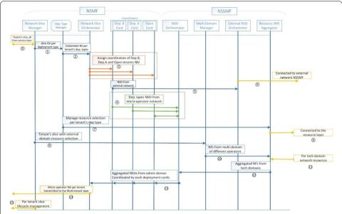
**Fig. 8** The message sequence diagram for the micro-operator network slicing MANO layer. This figure presents a sequence diagram from the operations in the Slicing MANO layer
