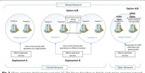
**Fig. 2** Micro-operator deployment scenarios [4]. This figure describes in details each micro-operator network deployment scenarios that can exist. This include the Open, Closed and Mixed micro-operator
