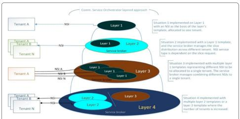
**Fig. 10** Communication service orchestrator implementation of multitenant-slice situation types. The figure presents the layers approach for achieving communication service distribution for each possible situation types that can exist
