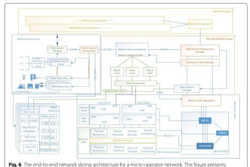
one of the main contribution in this paper which is the end-to-end network slicing architecture for a 5G micro-operator
