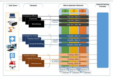
**Fig. 1** General micro-operator model [11]. This figure describes the overall model for a 5G micro-operator network considering all key elements such as the end users, tenants, verticals, and the micro operator network operator
