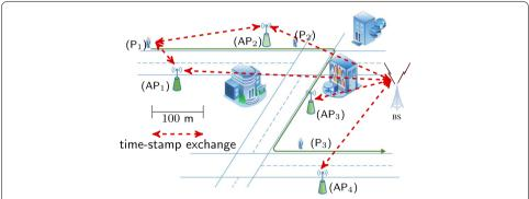
**Fig. 12** An example where MU joint sync&loc can be carried out. In each position, e.g.,  $P_1$ ,  $P_2$ , or  $P_3$ , the MU is exchanging time-stamps with at least two APs based on the protocol described in Sect. 2.3
