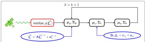
**Fig. 8** A summary of the BRF-based pairwise synchronization and joint sync&loc. The satellite information is used to initialize the joint sync&loc algorithm described in Sect. 5
