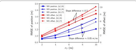
**Fig. 13** Impact of hybrid synchronization on MU joint sync&loc. (a)/(b) denotes the algorithm used for network synchronization (Sect. 4.1). The numbers in the legend denote the number of iterations each algorithm runs
