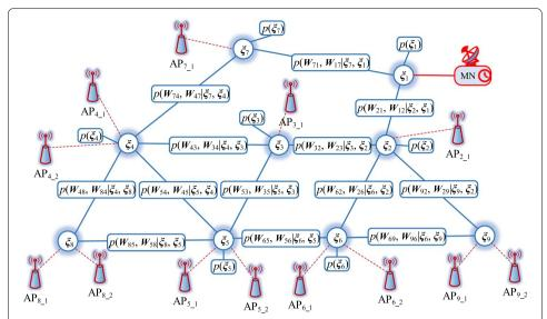
**Fig. 4** The FG corresponding to an exemplifying network. Note that, the FG is drawn only for the backhaul network to avoid unnecessary complexity. To draw the FG of the whole network, one can simply consider APs as variable nodes connected to their corresponding backhaul nodes via factor nodes
