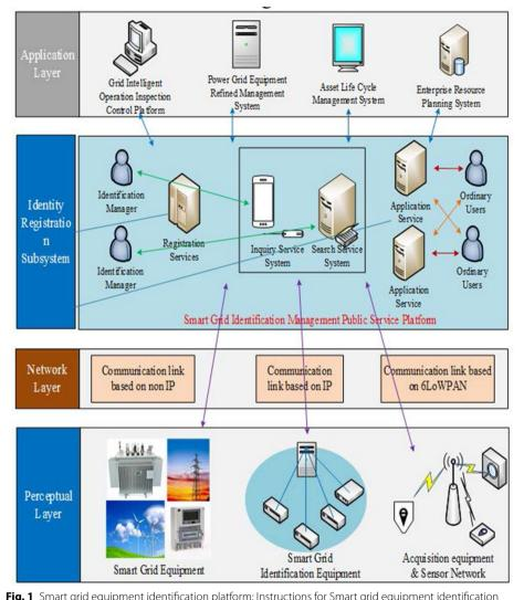
**Fig. 1** Smart grid equipment identification platform; Instructions for Smart grid equipment identification platform
