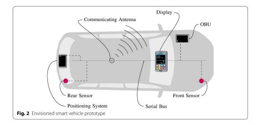
Dedicated Short-Range Communications (DSRC) protocol [81]. A Tamper Proof Device (TPD) is embedded in each OBU to store the user inaccessible cryptographic keying materials involved in cryptographic operations. Moreover, each vehicle has a unique barcode/identifier that can be known to the DOT. Figure 2 illustrates an envisioned smart vehicle prototype.
