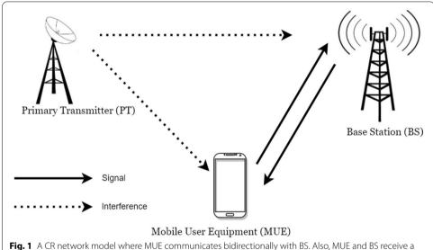
**Fig. 1** A CR network model where MUE communicates bidirectionally with BS. Also, MUE and BS receive a interference signal from PT
