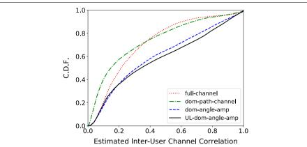
Fig. 3 The cumulative distribution function of estimated downlink inter-user channel correlation for all measured channels. This includes estimations by utilizing full downlink channel (labeled as full-channel), approximated downlink channel with downlink dominant angles (labeled as dom-path-channel), downlink dominant angles and amplitudes (labeled as dom-angle-amp), and uplink downlink dominant angles and amplitudes (labeled as UL-dom-angle-amp), respectively
